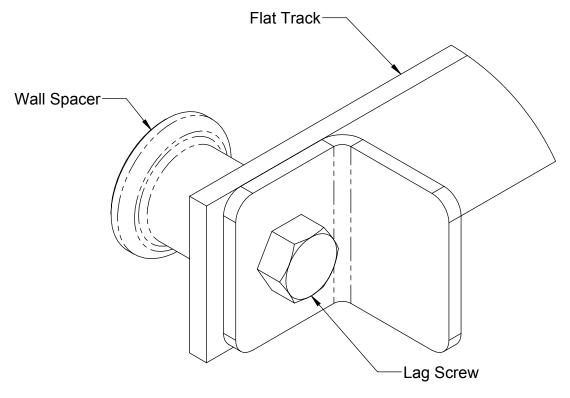
**Application:** The End Stop is used on each end of the Flat Track to stop the door hangers from falling off the ends of the track.
